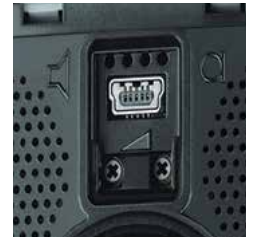
Mini-USB connection and loudspeaker/microphone volume adjustment
